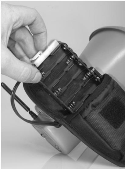
3. Orient the batteries as per the directions shown in each cavity within the holder. *Note that the battery polarity alternates.*
